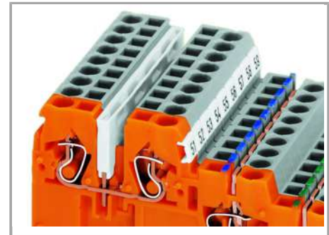
Commoning signal level voltage via insulated push-in type jumper bars (870 Series) – 2- to 9-way, depending on application.
