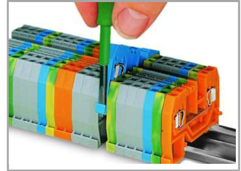
Removing a terminal block from the assembly.
