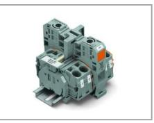
Step-down jumpers may common terminal blocks of different sizes, without losing a conductor clamping point. This can be beneficial on long conductor runs where voltage drops may be problematic. A large conductor can be easily connected to smaller conductors at the distribution point.
