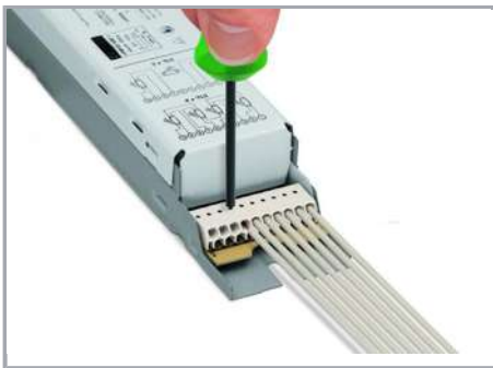
Removing a conductor via 1.0 mm Ø disconnection tool (206-841).
