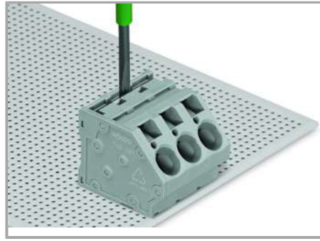
To insert a comb-style jumper bar, push it down using a screwdriver until it hits the backstop – 745 Series.
