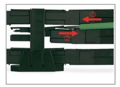
All distributor connections are locked and protected against accidental disconnection directly after mating. Locking of any connection is released using a screwdriver, even if all connections are in use.
