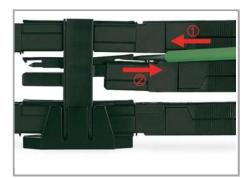
All distributor connections are locked and protected against accidental disconnection directly after mating. Locking of any connection is released using a screwdriver, even if all connections are in use.
