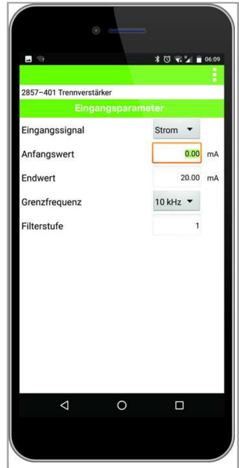
Configuration via WAGO interface configuration app
