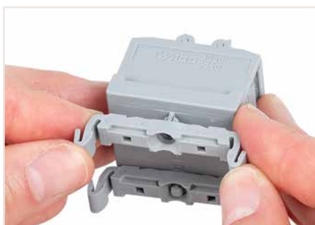
Terminal strip; with snap-in mounting feet Snapping a mounting foot (209-120). (Distance between mounting feet: approx. 20 ... 25 mm)
