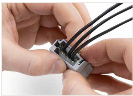
Close latch securely and press down in the center.
