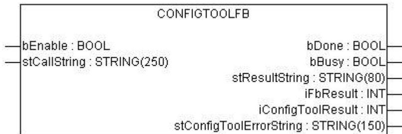
Figure 130: Graphical Representation of the “ConfigToolFB” Function Block
