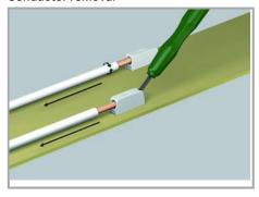
Use an operating tool or simply "twist and pull" to remove solid conductors.
