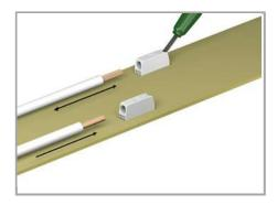
Insert fine-stranded conductors – and remove conductors – via operating tool. Solid conductors can also be terminated by simply pushing them in.
