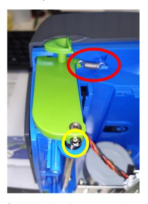
Red circle: Use pliers to remove the spring from the element.
