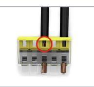
The transparent housing shows if conductors are fully inserted; within the colored base, a clear port shows if the conductor's strip length is correct. Conductors are correctly stripped if the clear port shows no bare conductor on the unprinted connector side. Picture shows center conductor with exceeded strip length.
