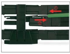
All distributor connections are locked and protected against accidental disconnection directly after mating. Locking of any connection is released using a screwdriver, even if all connections are in use.
