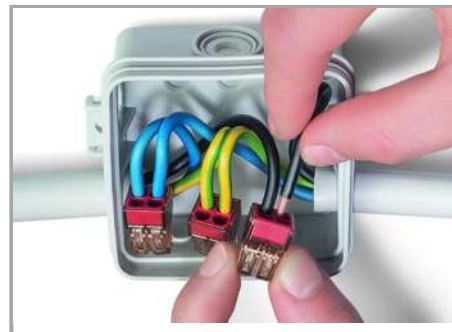
Termination: Insert stripped solid conductor until it hits backstop.
