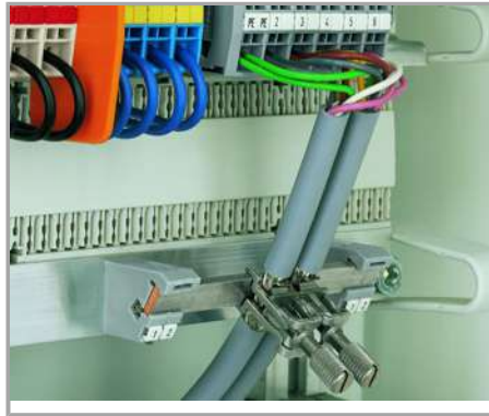
Insulated mounting carriers for a common shield reference potential, independent of housing potential
