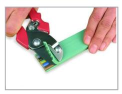
Cut off the flat cable insulation via cable cutter.
