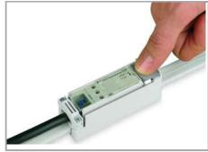
Insert upper part into base until it hits the stop (which will click when engaged). Push down and lock lever. All three cores are contacted simultaneously.
