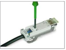
Cut outgoing feeder cable, completely strip and insert conductors. Tighten screws firmly (observe 0.7 Nm of tightening torque).
