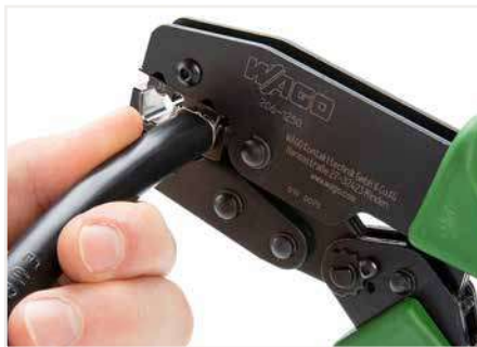
Squeeze handles until ratchet mechanism is released.
