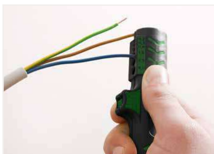
Stripping the conductor insulation.
