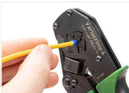
Squeeze handles until ratchet mechanism is released.
