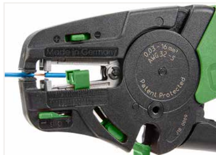
Partially stripping a conductor.
