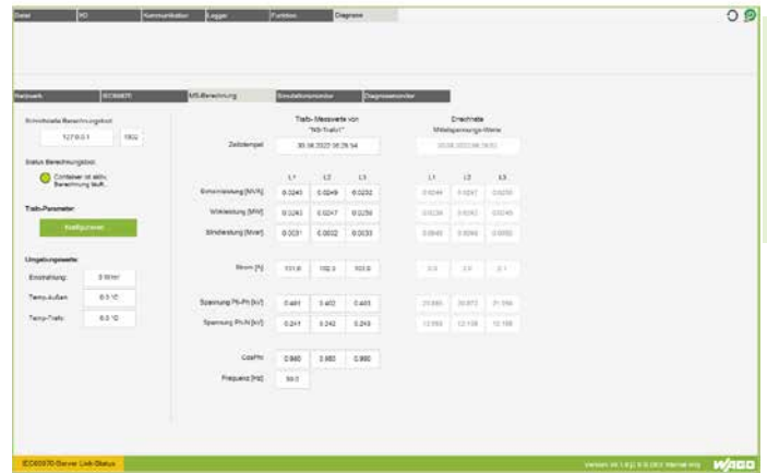
View of the current measured values and the calculated medium voltage values
