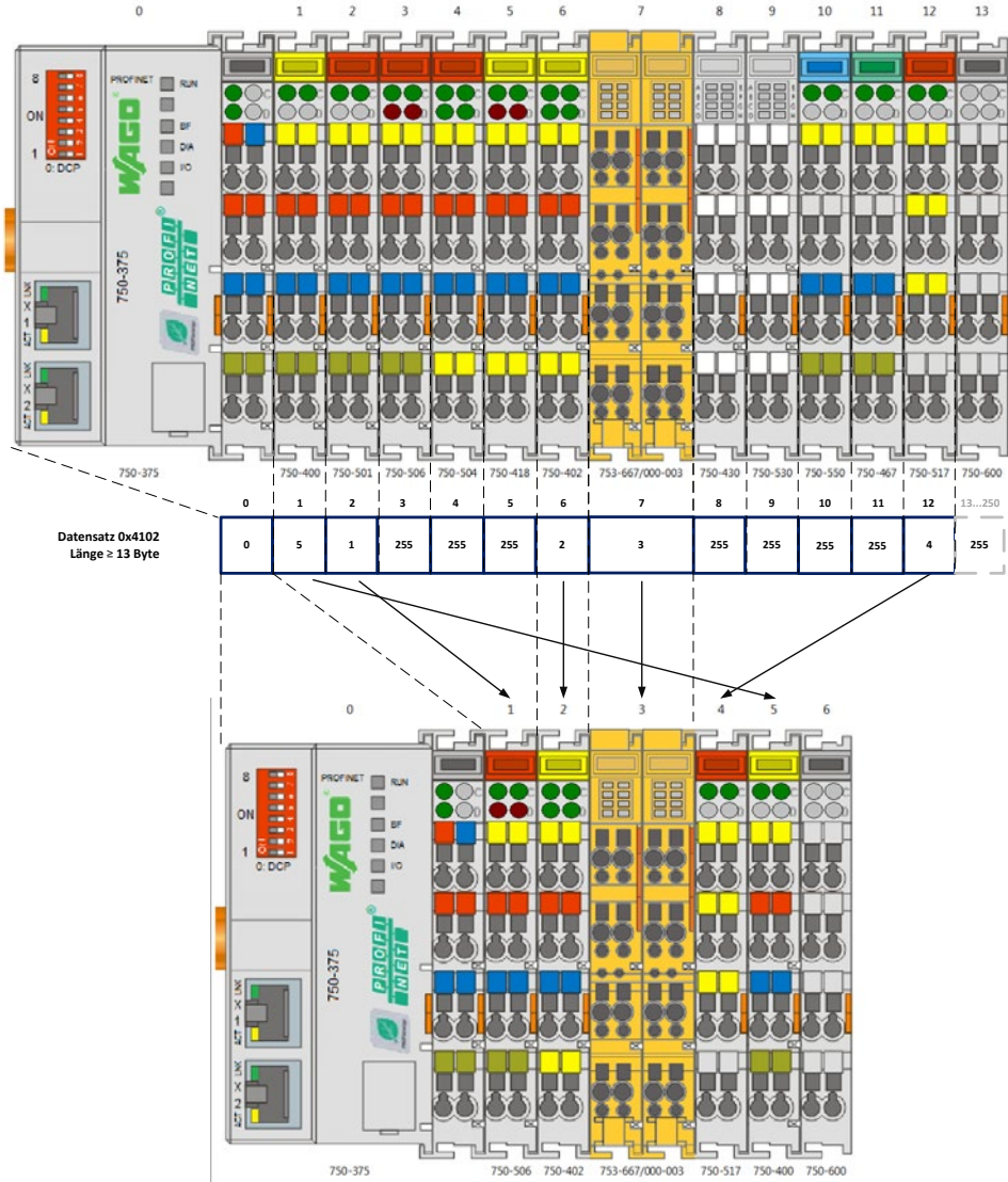
Figure 51: Mapping the Projected Station Layout onto the Physical Layout
