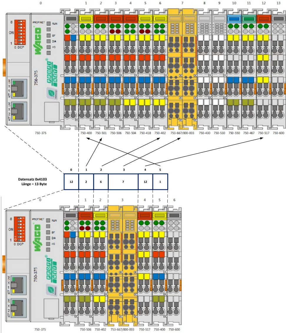
Figure 52: Mapping a Physical Station Layout onto the Projected Station Layout
