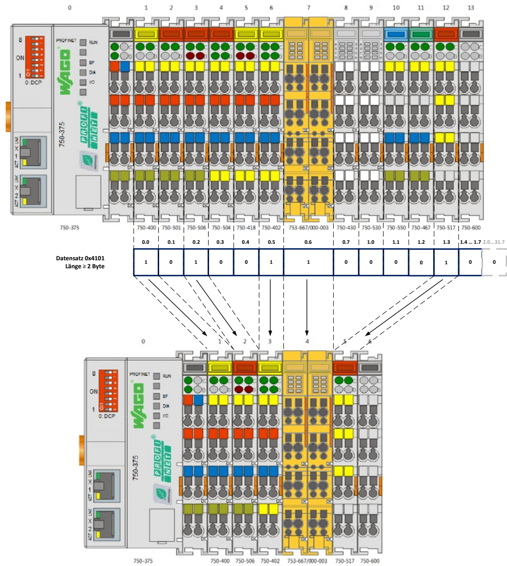
Figure 50: Bitwise Activation of the Slots (Example)
