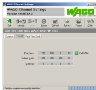
Fig. 3-2: Setting IP addresses using WAGO ETHERNET Settings
