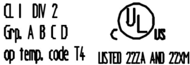
Fig. 9.5.2-4: Printing on text detail in accordance with CENELEC and IEC
