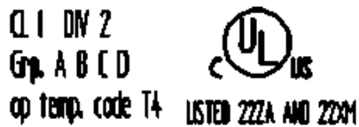
Figure 91: Printing on text detail in accordance with NEC
