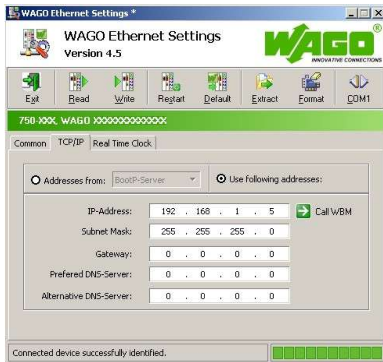
Figure 45: Setting IP addresses in WAGO-ETHERNET-Settings
