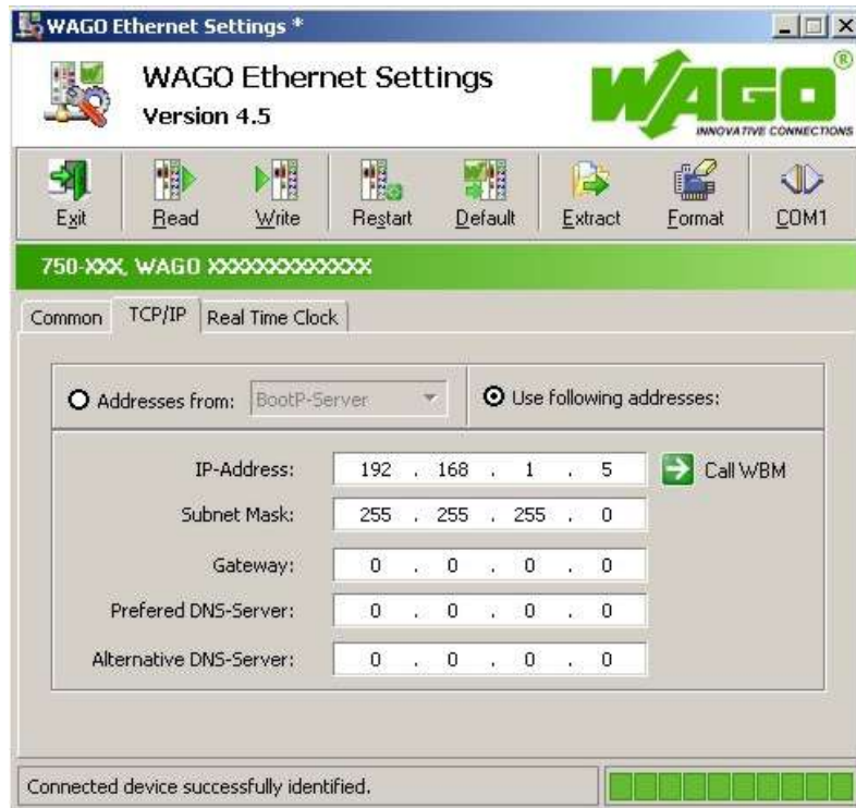
Figure 46: Setting IP addresses in WAGO-ETHERNET-Settings
