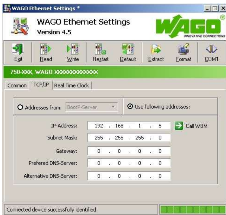
Figure 48: Setting IP addresses in WAGO-ETHERNET-Settings
