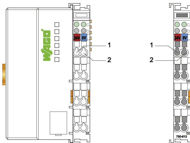
Figure 6: System Supply via Fieldbus Coupler/Controller (left) and via Internal System Supply Module (right)
