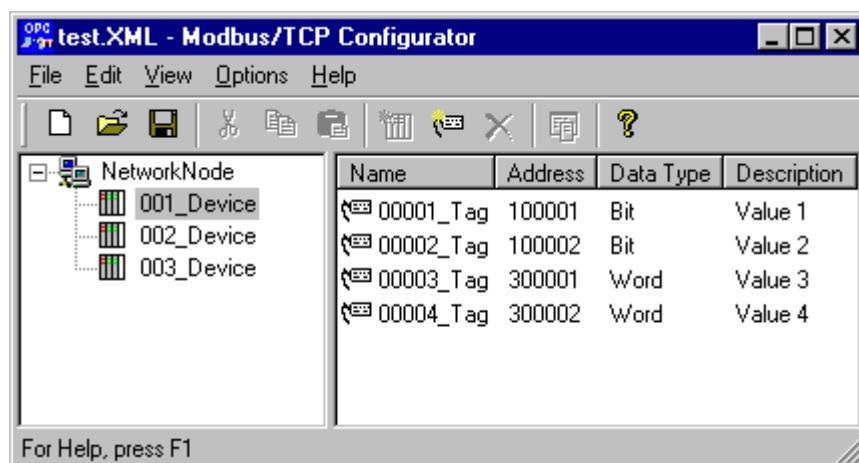
The configurator is structured in the same way as the Windows Explorer. The window of the configuration application consists of two parts. The left part contains the Modbus/TCP devices of the system in tree topology . In the right part, the process values (tags) possible with OPC which belong to the device currently selected in the device tree are listed.
