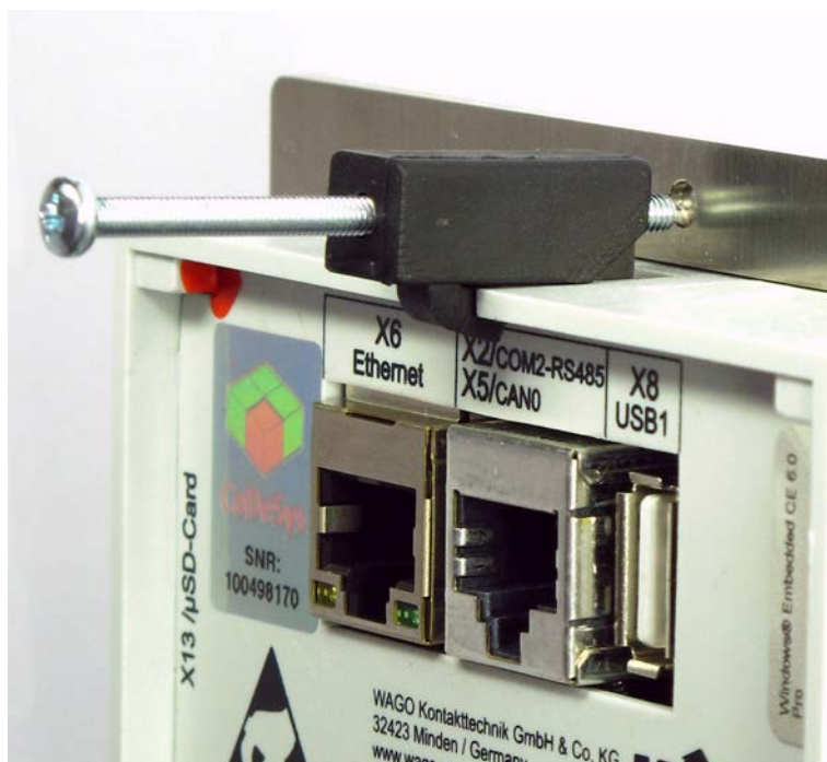
Figure 9: Detailed Photograph of Installation with Intermediate Plate
